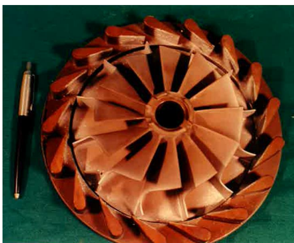
Figure 1: A view of radial inflow turbine hardware and diagram indicating the fluid flow
