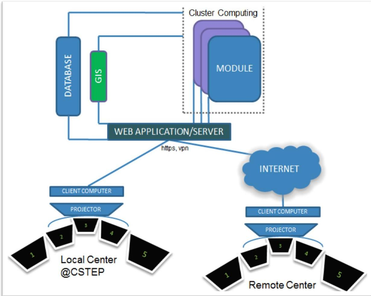
**Figure 20 : System Architecture**
