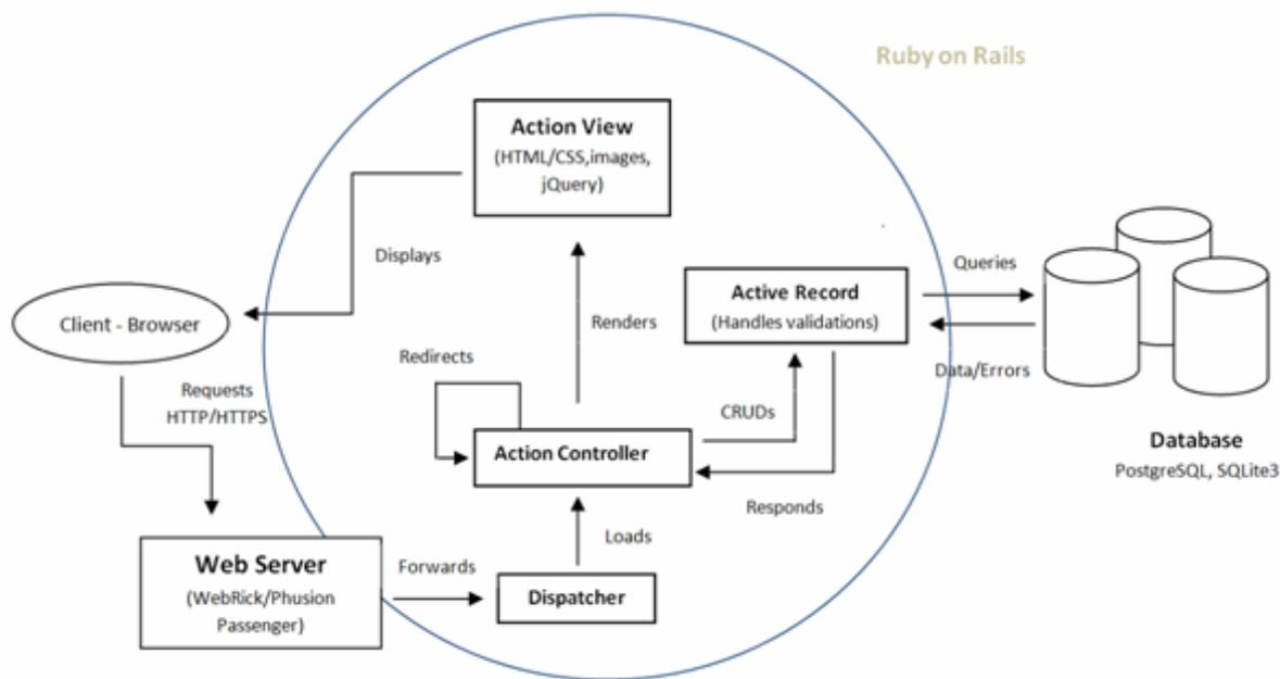
Figure 19 : Ruby on Rails – MVC Architecture
