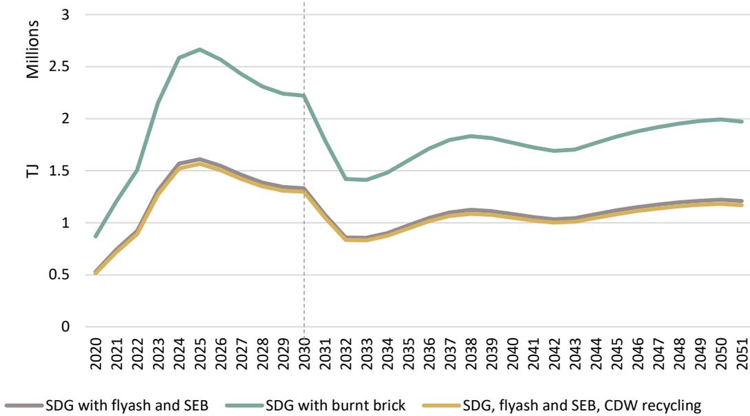
Figure 32 Annual embodied energy from housing construction under various construction material combinations
