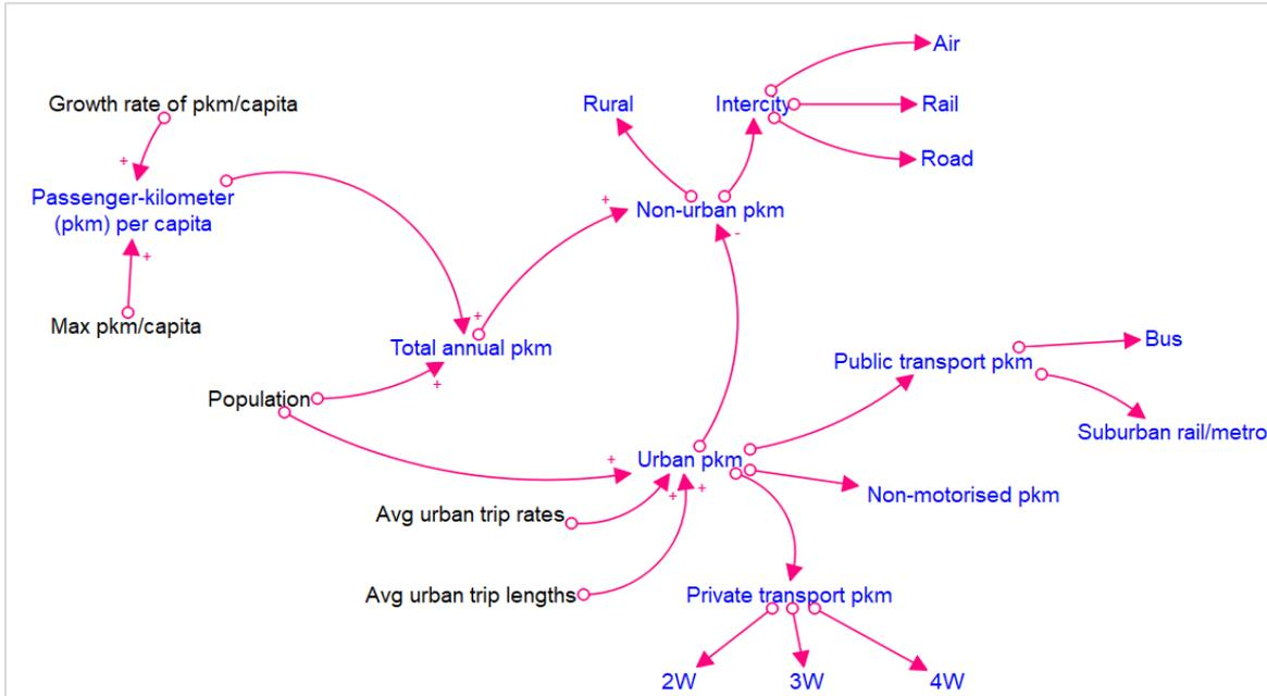
Figure 11: Passenger transport causal loop diagram
