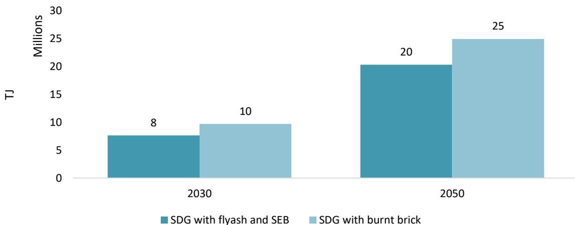
Figure 33 The cumulative embodied energy of cement used in construction under various scenarios
